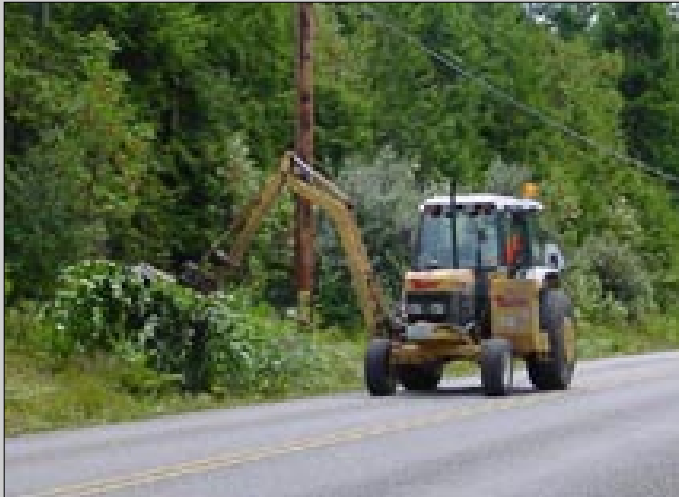
Brushing machines are used to control woody plants, such as the alder that has been leveled here. The machine takes the tree down in the first pass and mulches it in the second.
