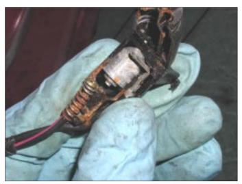
Hood-light and trunk-light switches in pre-1998 vehicles often contain mercury. These switches are usually easily replaced with non-mercury, ball-bearing switches.
