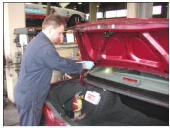
The next time you have your vehicle in for service, have the mechanic check the hood- and trunk-light switches, and replace them if they contain mercury.
