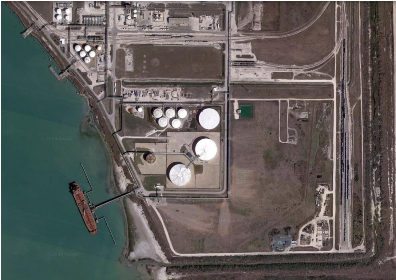
Occidental Petroleum's chemical production facility on Corpus Christi Bay is a major supplier of vinyl chloride to PVC plants throughout the Americas, from Canada to Colombia. It delivers vinyl chloride in refrigerated boats (seen at left) and rail tank cars (seen at right). Google Earth photo .
